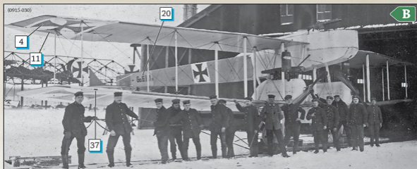
Gotha G.1 11/15 is seen here armed with two LMG 14 Parabellum machine guns but does not appear to be carrying any bombs in its fairing. Note the pale blue(?) underside colour of the wings. The top leading edge and tips of the top wing appear to remain in their original field grey finish. The leading edge and tips of the bottom wings appear to have been overpainted in an even darker colour, perhaps black. See also page 19.
