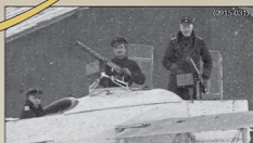
Modified cockpit coaming and cupola gun ring detail from Gotha G.1 11/15 B. Note the twin LMG 14 Parabellum machine guns and magazines.
